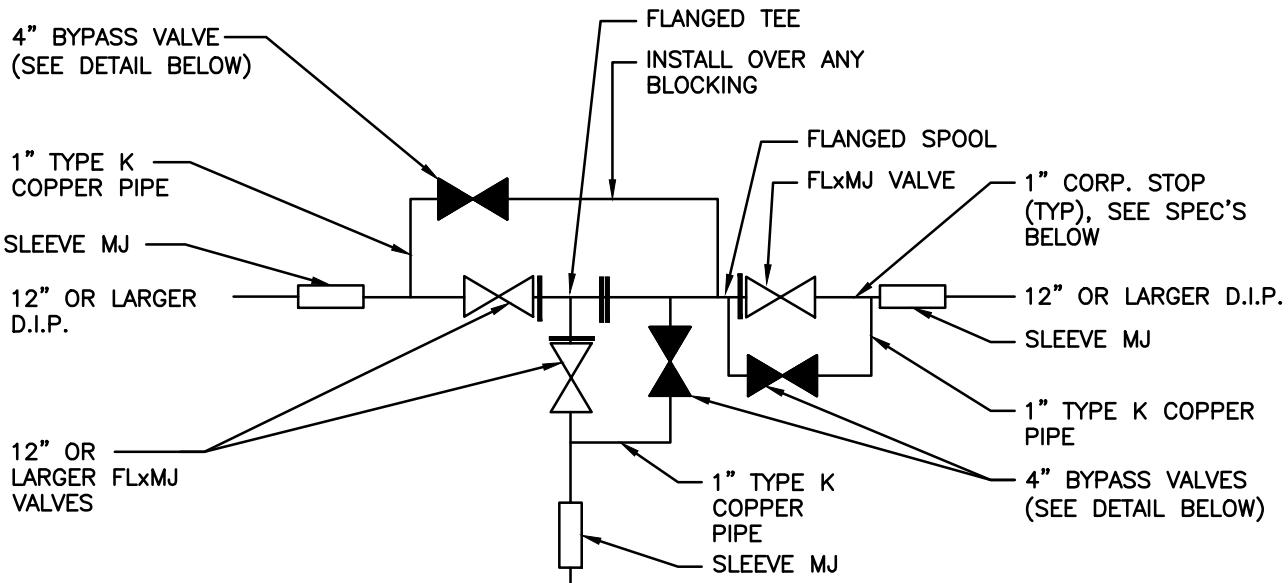
NOTE: BYPASS VALVE SHALL BE USED WHEN STATIC WATER PRESSURE EXCEEDS 150 P.S.I ON WATER MAINS 12" AND LARGER, AS DIRECTED BY THE DISTRICT.
