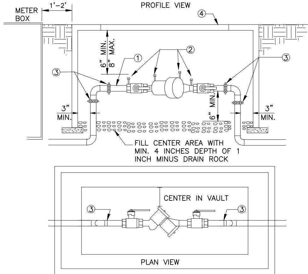
\* DCVA-BOX SHALL BE LOCATED IMMEDIATELY DOWNSTREAM OF WATER METER BOX PRIOR TO AND BRANCH CONNECTIONS. WITH NO MORE THAN 1'-2' BETWEEN BOXES.
