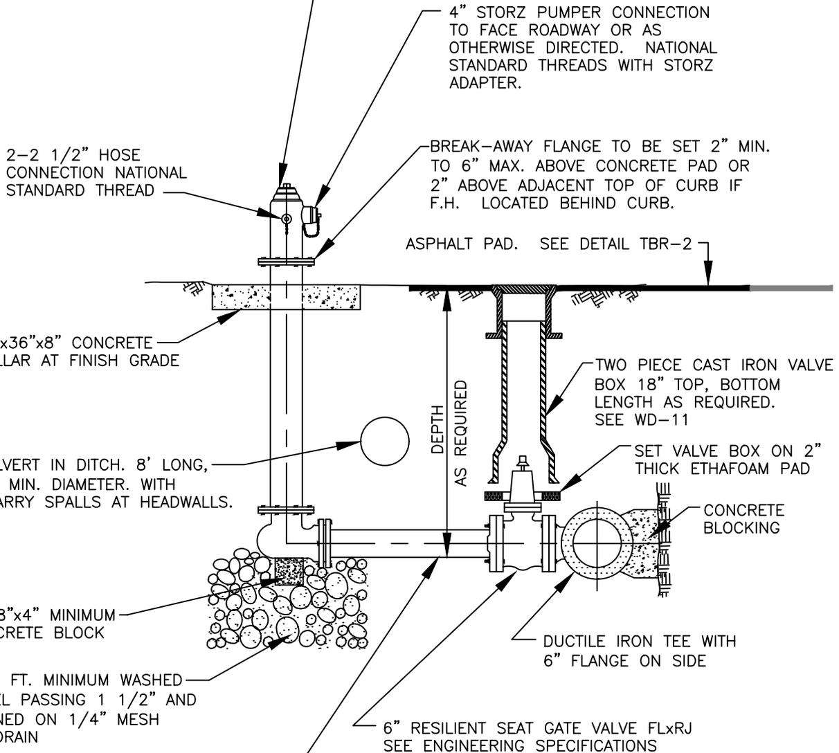
6" DUCTILE IRON CLASS 52 PIPE WITH POLY WRAP AND RESTRAINED JOINTS ENTIRE LENGTH, INCLUDING VALVE AND HYDRANT BEND.
